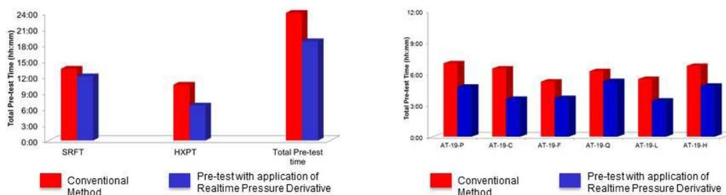
Figure B – (Left) AE well, example, total pressure test time comparison between conventional method and pre-test by using realtime derivative pressure which is saved operation time about 5 hours. (Right) Arthit infill development wells, example, total pressure test time comparison between conventional method and pre-test with realtime derivative pressure which is totally saved operations time about 12 hours.
