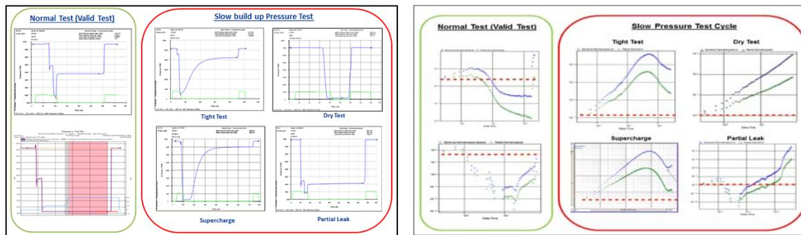
Figure A – (Left) Pressure versus time plot in each type of pressure test in conventional. (Right) Realtime derivative pressure, valid test (normal test) need to pass wellbore storage which the end of pressure derivative point is below the first point (below dash line). In slow build up pressure test, realtime pressure derivative are not pass wellbore storage except partial leak.
