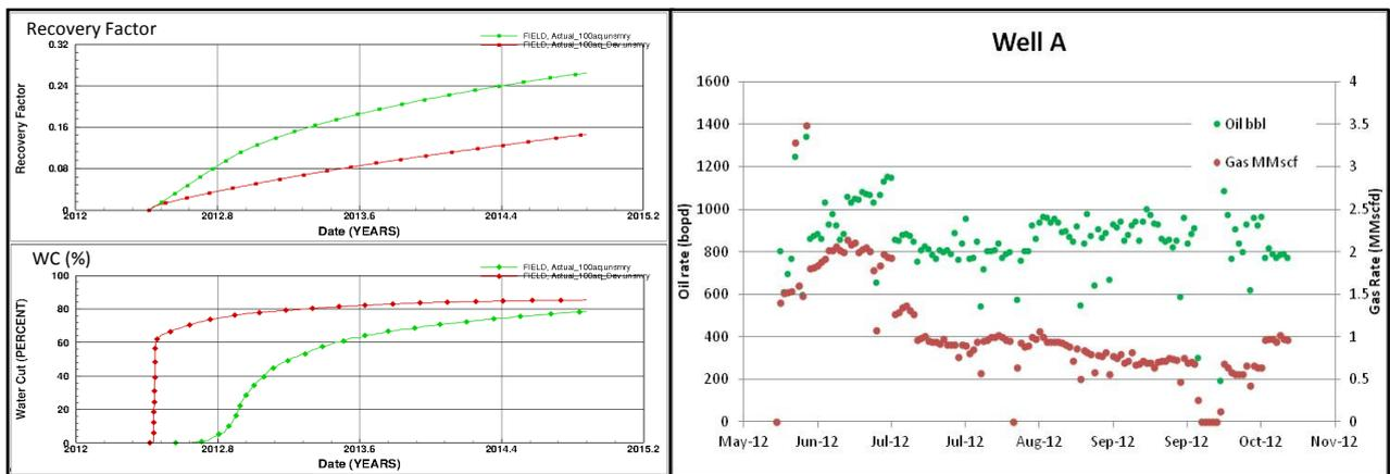
Figure 4: Simulation result compare between horizontal well (green line) and deviated well (red line) performance, (top) recovery factor, (bottom) Water cut.
